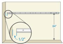
\* Rails are typically mounted at 94" when incorporating a Double-Hang O-Box.
